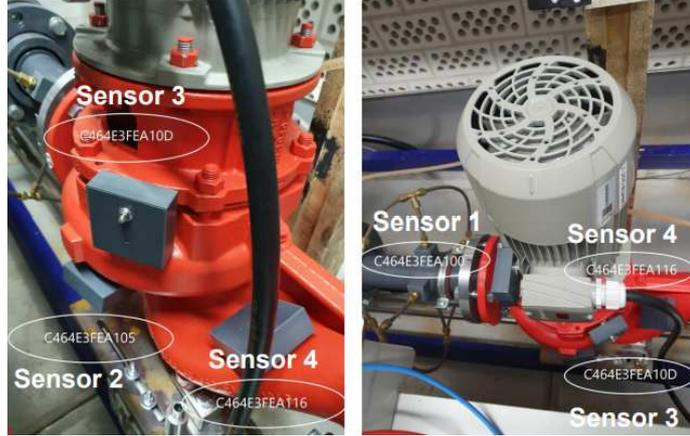
Figure 3.1: Pump and sensor setup
